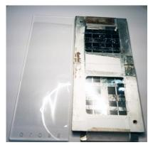
**2. Thermal evaporation of Source and Drain contacts.** Use a thermal evaporator to deposit 35 nm-thick silver (Ag) source and drain contacts.
