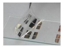
**3. Thermal evaporation of the Gate electrode.** After depositing the Source and Drain contacts, deposit silver Gate electrode (35 nm-thick) on the opposite side of Mylar. The gate shadow mask must be aligned correctly to completely overlap the area between the contacts (the channel area).
