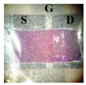
**9. Device wiring.** Attach thin gold wires to the silver Source, Drain and Gate electrodes using a silver paint. Let the paint dry in the dark. The device is ready for wiring to your measurement setup. Contacting the device with external pins of a probe station instead of using wires is also possible.
